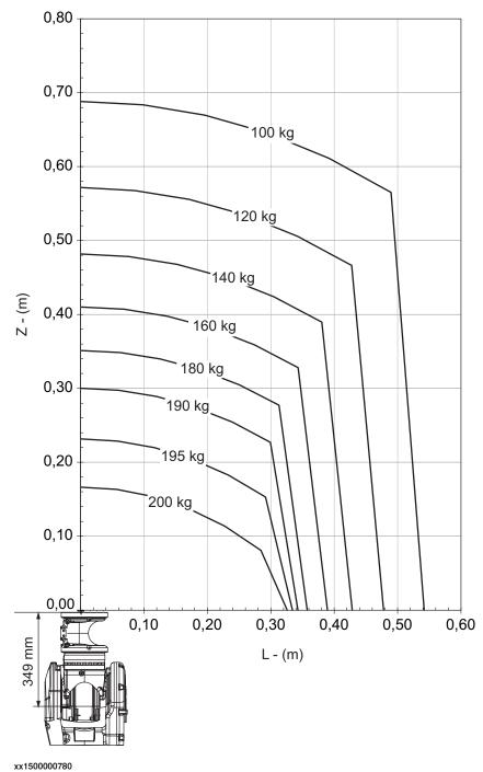
1.5.3 Maximum load and moment of inertia for full and limited axis 5 (center line down) movement
